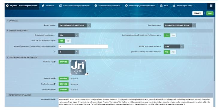
**1** The TUR (Test Uncertainty Ratio) is the MPE/Incertitude ratio. This calculation indicates the ability of the measurement chain to respond to measurement uncertainties.
