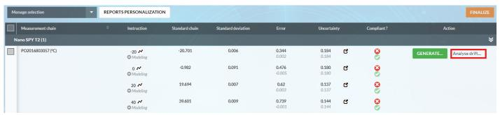
• Choosing an adjustment action following a calibration or verification sends a modelization command to the device. Only compatible connected devices can be adjusted. No adjustment is possible on generic measuring chains.
